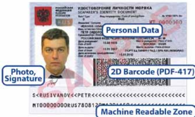
General view of SID according to the ILO SID-0002 Technical Standard
